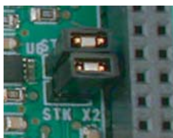
Figure 2-8 . STKX1 and STKX2 jumpers on STK526
