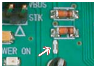
Figure 2-10 . Configuration Pad Location
