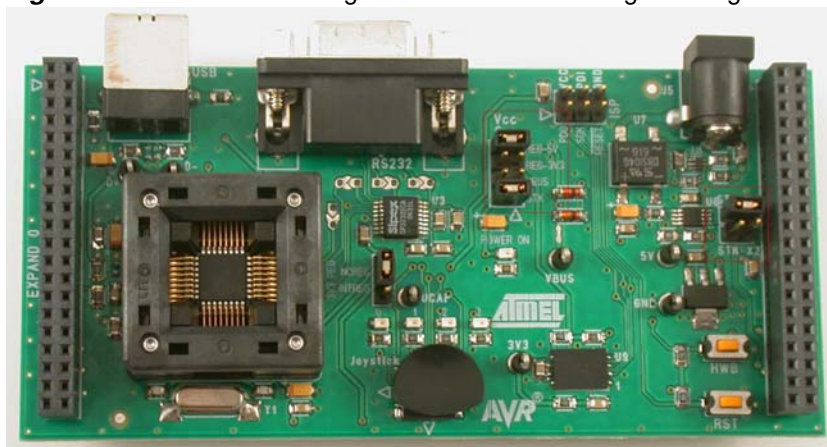
Figure 2-25 . STK526 Configuration for Parallel Programming
