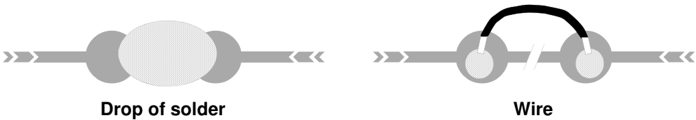
Figure 2. Configuration Pad - Re-connection
