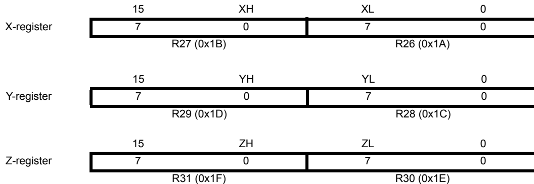
Figure 4-3. The X-, Y-, and Z-Registers
