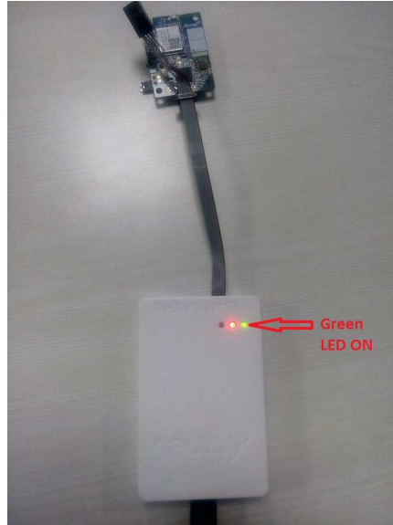
Figure 3-4. Atmel-ICE 10-pin Header Orientation
