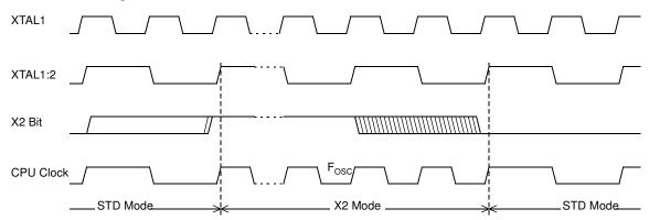
The X2 bit in the CKCON0 register (see Table 7-1) allows a switch from 12 clock periods per instruction to 6 clock periods and vice versa. At reset, the speed is set according to X2 bit of Hardware Security Byte (HSB). By default, Standard mode is active. Setting the X2 bit activates the X2 feature (X2 mode).
