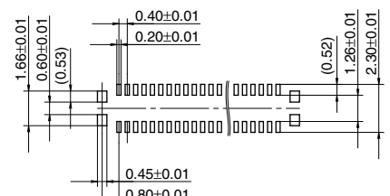
Recommended metal mask pattern Metal mask thickness: When 120μm (Terminal opening ratio: 70%) (Metal-part opening ratio: 100%)
