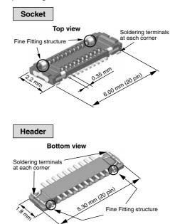
Proprietary Fine Fitting construction High unmating force is maintained while soldering terminals on socket and header are held in place. Soldering terminal on header Soldering terminalt on socket
