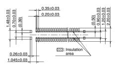
Recommended metal mask pattern Metal mask thickness: When 100µm (Signal terminal opening ratio: 70%) (Power terminal opening ratio: 77%)
