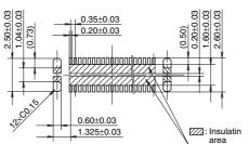
Recommended metal mask pattern Metal mask thickness: When 100µm (Terminal opening ratio: 70%) (Metal-part opening ratio: 46%)
