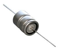
Type AXLH capacitors are a new generation of high performance aluminum electrolytic capacitors rated up to 2000 hours at 150 °C. They are designed for applications that place high demands on a capacitor. The capacitor's outstanding features include low ESR, low leakage current, a long shelf life and a high ripple current capability.
