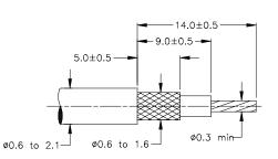
For best results, stripped cable should meet the dimensions given here.
