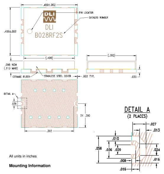
PCB ground pattern length and width can be 0.002-0.003 inches larger than filter footprint. Dimensions of filter launch and PCB launch pattern should be closely matched.
