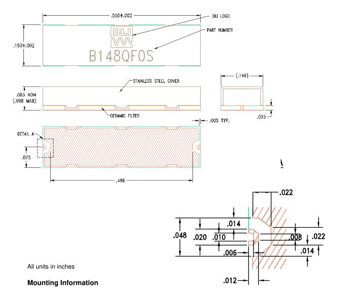
PCB ground pattern length and width can be 0.002-0.003 inches larger than filter footprint. Dimensions of filter launch and PCB launch pattern should be closely matched. It is suggested that PCB ground metal be pulled back from RF I/O trace to account for component alignment tolerance. Ground via depth and spacing should be set so as not to create any resonances at the frequency of operation. Reference SMT Filter Mounting application note for additional mounting information.
