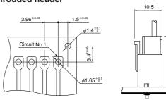
\*11.0 max. when used with the VR connector receptacle.
