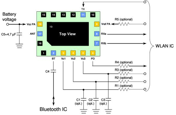
All RF ports are 50 Ohm matched. WLAN RX ports are matched to 100 Ohm differential impedance. All RF ports except for Bluetooth RX/TX are internally DC-decoupled. For the Bluetooth port an external DC-decoupling capacitors may be required (this pin is coupled with DC voltage).
