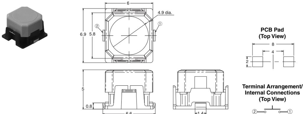
**Note:** Unless otherwise specified, a tolerance of ±0.4 mm applies to all dimensions. No terminal numbers are indicated on the Switches.
