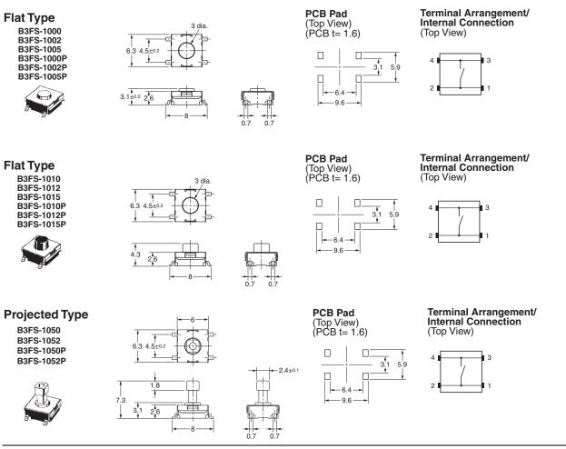
Note: Unless otherwise specified, a tolerance of ±0.4 mm applies to all dimensions. No terminal numbers are indicated on the Switches.
