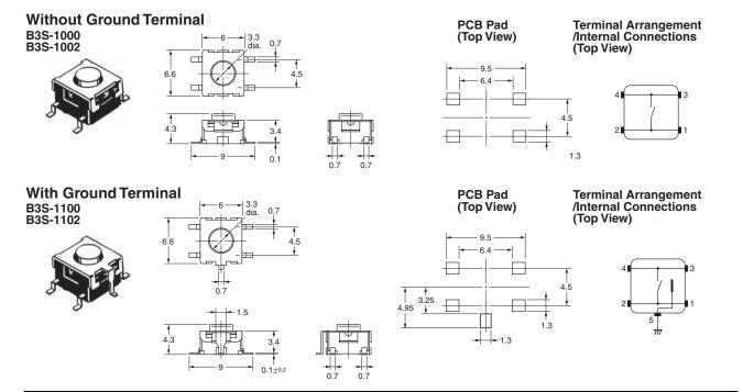
Note: Unless otherwise specified, a tolerance of ±0.4 mm applies to all dimensions. No terminal numbers are indicated on the Switches.
