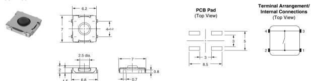
Note: Unless otherwise specified, a tolerance of ±0.4 mm applies to all dimensions. No terminal numbers are indicated on the Switches.
