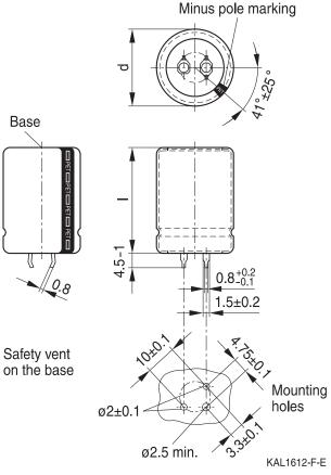
Snap-in capacitors are also available with 3 terminals (length (4.5-1) mm). PET insulation is marked with "PET" on the sleeve.
