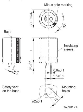
Snap-in terminals, length  $(6.0\pm1)$  mm. Also available in a shorter version with a length of (4.5-1) mm. PET insulation is marked with "PET" on the sleeve.
