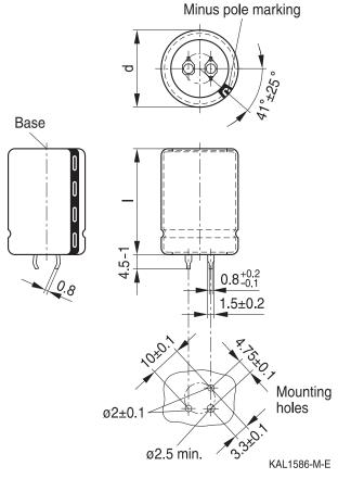
Snap-in capacitors are also available with 3 terminals (length (4.5-1) mm). Safety vent on the base.
