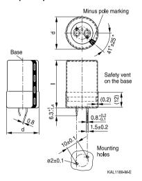
Snap-in terminals, length (6.3 + 1/-1.4) mm. Also available in a shorter version with a length of (4.5 - 1.4) mm. PET insulation cap is positioned under the insulation sleeve.
