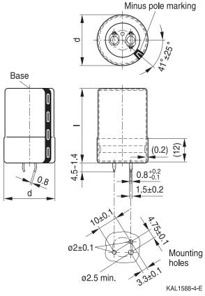
Snap-in capacitors are also available with 3 terminals (length (4.5-1.4) mm). PET insulation cap is positioned under the insulation sleeve. Safety vent on the case wall.
