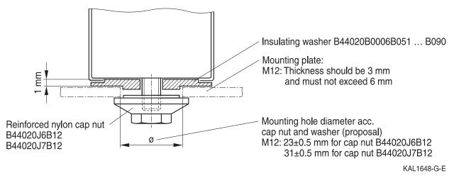
Mounting stud has the same potential as the negative terminal. Attention must be paid on any relevant regulations (e.g. VDE, BSA or UL).
