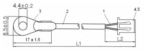
Dimensions in mm, Tolerances acc. to ISO 2768-m unless specified
