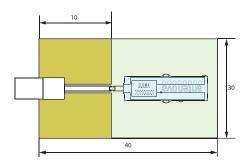
The testboard is designed for evaluation purposes for Flavus antenna. The card has the same size as a typical PCMCIA card and is fitted with an SMA connector.
