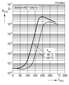
$\begin{array}{l} \mbox{PTC resistance $R_{PTC}$} \\ \mbox{versus PTC temperature $T_{PTC}$} \\ \mbox{(measured at low signal voltage)} \end{array}$
