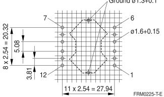
Hole arrangement View in mounting direction (Note half pitch!)
