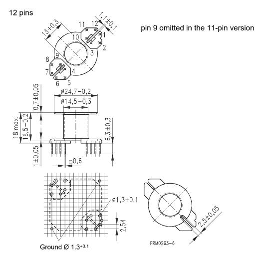
Hole arrangement View in mounting direction
