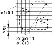
Hole arrangement View in mounting direction
