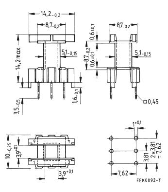
Hole arrangement View in mounting direction
