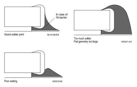
Good and poor solder joints caused by amount of solder in infrared reflow soldering
