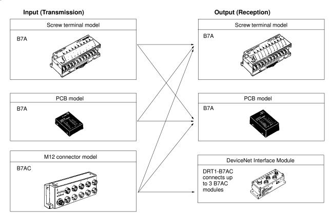
Note: The 10-point model has a normal I/O delay of 19.2 ms (typical); 10-point models with short I/O delay are not available.
