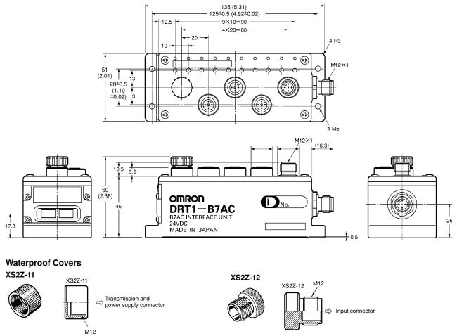
Note: The B7AC maintains IP67 with the XS2Z-11 and XS2Z-12 Waterproof Covers. Be sure to connect the XS2Z-11 and XS2Z-12 Waterproof Covers to the connectors by hand and tighten the Waterproof Covers securely with a force of 4 to 5 kgf • cm (0.39 to 0.49 N • m).
