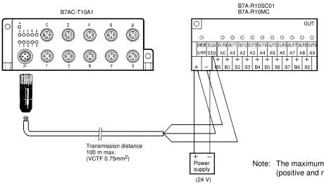
Note: The maximum current flow of the power lines (positive and negative lines) is 1.2 A max.
