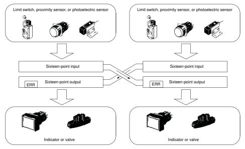
Note: The B7AM transmits input signals from SIG1 (input terminal) to SIG2 (output terminal). If an error results while the B7AM is transmitting input signals, an error signal is output from the output side only.
