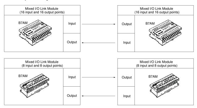
Note: The Mixed I/O Link Modules are either 3 ms (typical, for high-speed models) or 19.2 ms (typical, for normal-speed models). Use a Mixed I/O Link Module with the same transmission speed (I/O delay time).
