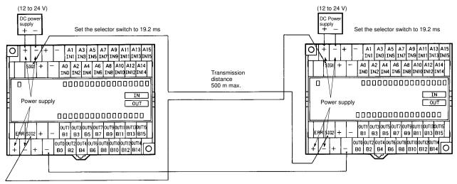
Note: A twisted pair or VCTF cable with a thickness of 0.75 mm<sup>2</sup> min. must be used for signal transmission.
