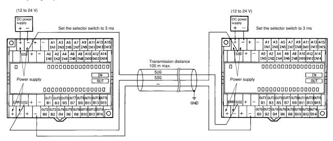
Note: A shielded cable with a thickness of 0.75 mm<sup>2</sup> min. must be used for signal transmission. It is recommended that the shield be grounded.
