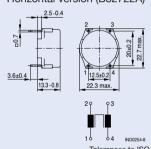
Tolerances to ISO 2768-C unless otherwise noted. Dimensions in mm.
