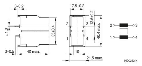
Part tolerances to ISO 2768-cL / ISO 8015. Size ISO 14405 © All dimensions in mm
