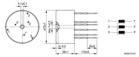
Dimensions in mm Tolerances acc. ISO 2768-c
