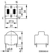
General tolerances according to ISO 2768-cL Dimensions in mm
