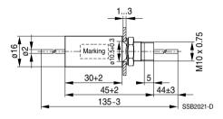
Tightening torque: 3 +0.5 Nm
