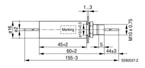
Tightening torque: 3 +0.5 Nm
