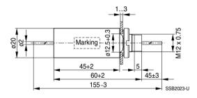
Tightening torque: 4 +0.5 Nm
