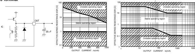
Fig.32 Output Equivalent Circuit
