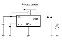
Fig.35 Bypass diode
