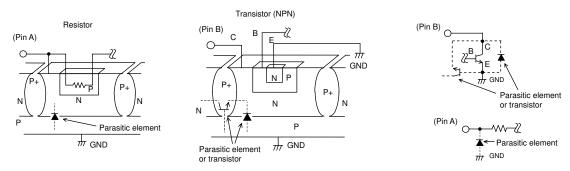
Fig.36 Example of the basic structure of a bipolar IC
