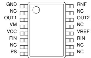
Fig.30 BA6285FS (SSOP-A16)
