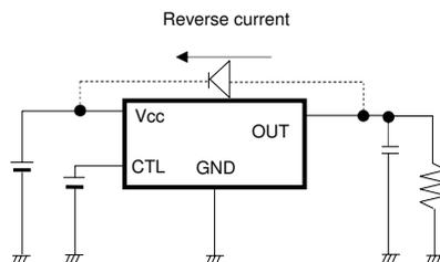
Fig.35 Bypass diode
