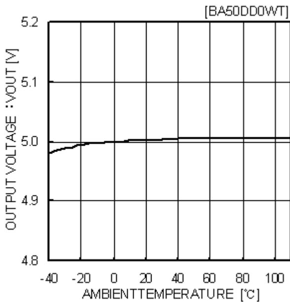
Fig.21 Temperature Characteristics
