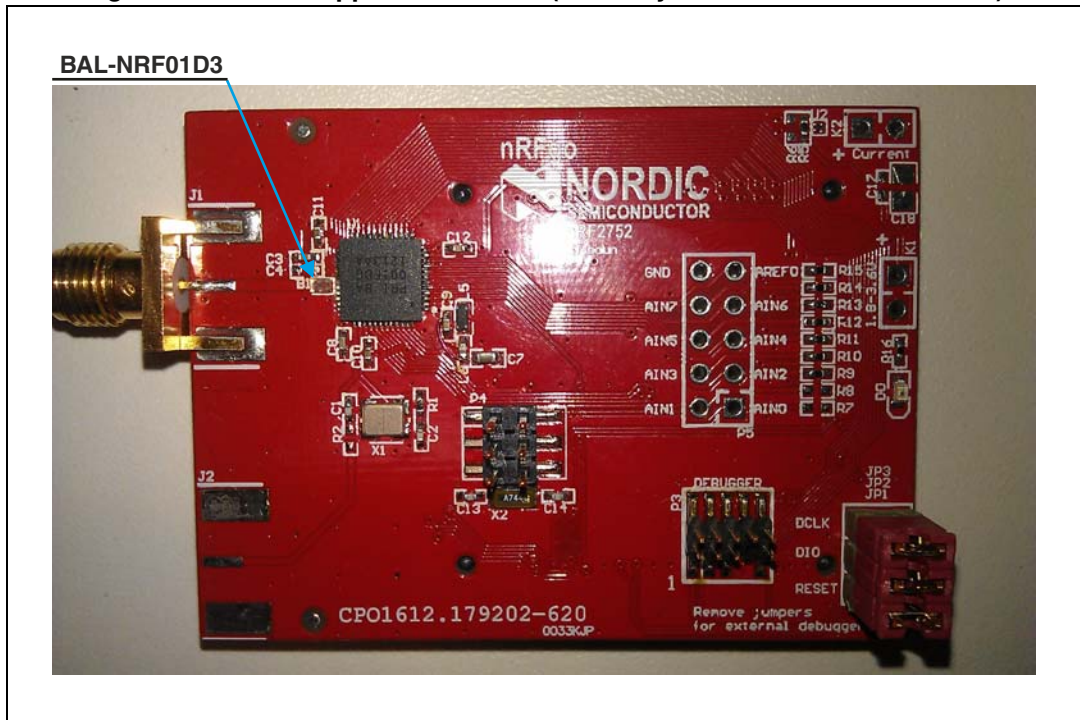
Figure 9. nRF2752 application board (courtesy of Nordic Semiconductor)
