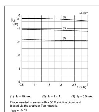
Fig.4 Insertion loss  $|s_{21}|^2$  of the diode in on-state as a function of frequency; typical values.
