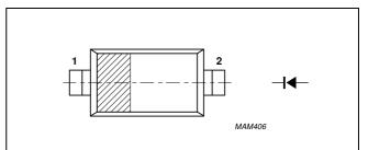
Marking code: A7 The marking bar indicates the cathode.
