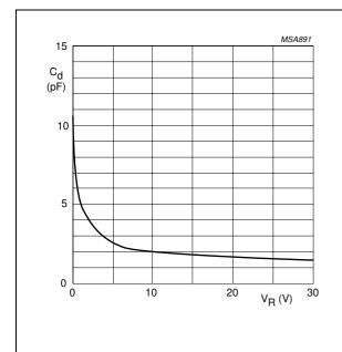
f = 1 MHz;  $T_{amb} = 25 \,^{\circ}\text{C}$ .
