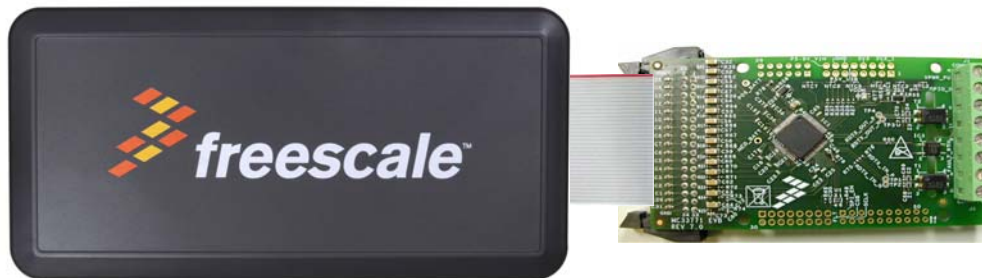
Figure 6. BATT-14AAAPACK Connection to KIT33771TPLEVB
