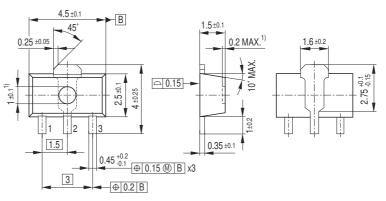
1) Ejector pin markings possible
