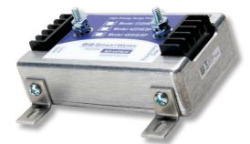
These three-stage surge protectors protect against lightning strikes, power surges, and other types of voltage disturbances with three stages of protection for each line: a gas discharge tube followed by a series resistor and finally a Transient Voltage Suppresser (TVS).
