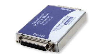
Model 422CEC, RS-232 to RS-422 converter, converts unbalanced RS-232 signals to balanced RS-422 signals. The RS-422 Standard uses a balanced voltage digital interface to allow communications of 90K bits per second on cable lengths of 4000 feet. If this baud rate is exceeded the line length will decrease accordingly. Ten receivers can be connected to any one driver for use in multidrop systems.
