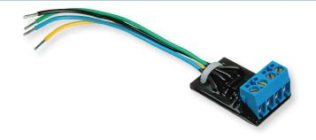
Single stage surge protectors offer a high degree of protection with Transient Voltage Suppressors (TVS) for each protected line.
