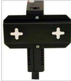
The IE-MultiWay can be mounted with two DIN Rail clips, a hardware option available through B+B SmartWorX. The DIN Rail clips include screws, to allow the installation onto a DIN Rail. Install the screws into DIN Rail clips, which can be mounted parallel or perpendicular to the DIN Rail. Snap the converter onto the clips. To remove the converter from the DIN Rail, use a flat-head screwdriver into the slot to gently pry the converter from the rail. Refer to picture on page 7.
